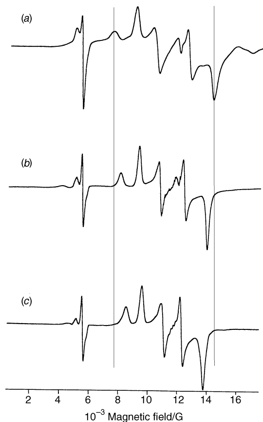
Fig. 4 Q-Band EPR spectra of [\{\text{CuL}(\text{NO}_3)_2\}_2][\text{NO}_3]_2 at (a) 300, (b) 160 K and (c) 4.2 K. The vertical lines are drawn to highlight the decreasing spread of the |\Delta M_S| = 1 resonances with temperature which shows that there is a decrease in the zero-field splitting
